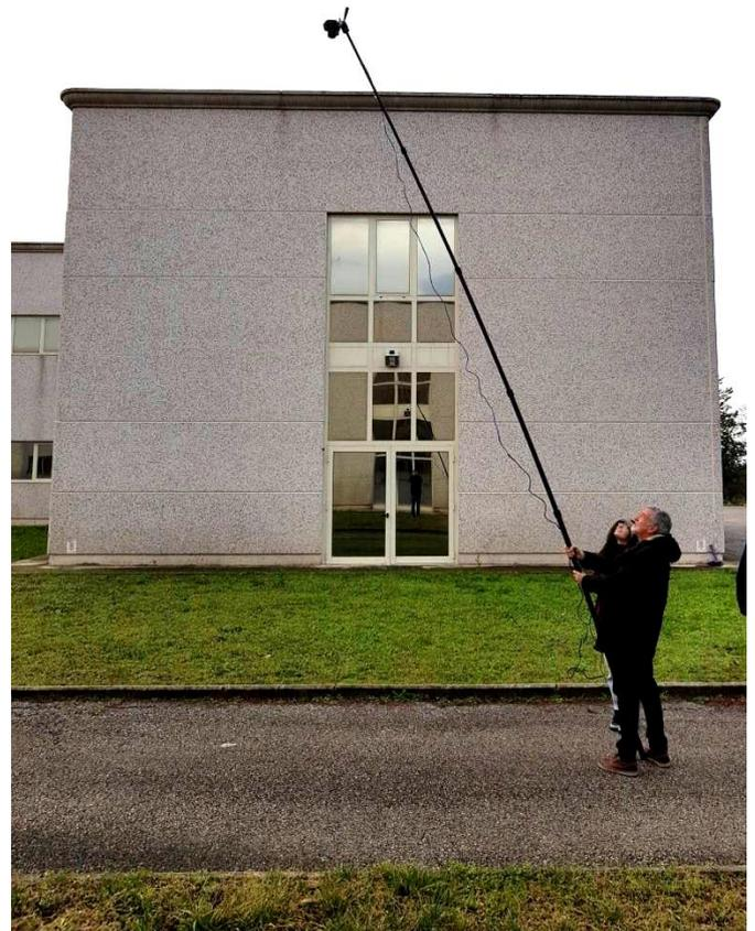
Figure 7. Fanotec carbon pole used for testing the GSD of a reflex camera at different heights.
