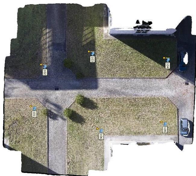
Figure 5. Ortho-rectified image of a flat surface improved with total station measurements.
