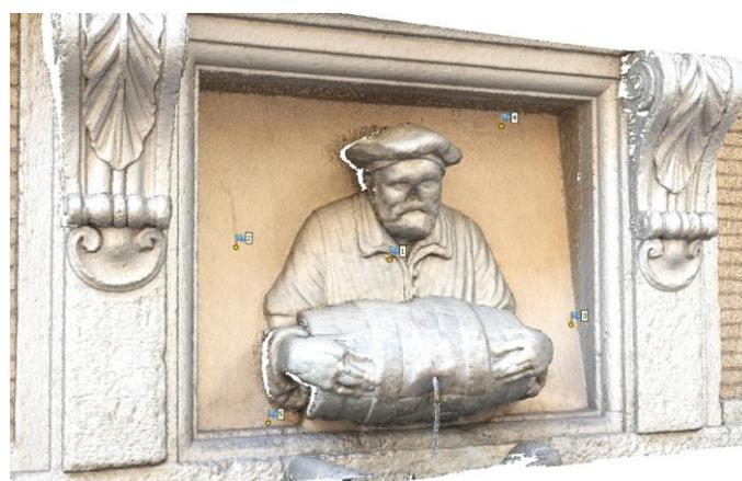
Figure 2. Dense cloud generated from photomodeling system with a 50 mm optic lens and 5 GCPs identified on the numerical model.
