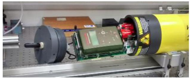
Figure 5. Detail of an autonomous recorder used for the calibrations, with the hydrophone and end cap removed from the main body showing the internal recording device. Body dimensions are approximately 16 cm diameter by 80 cm length.
