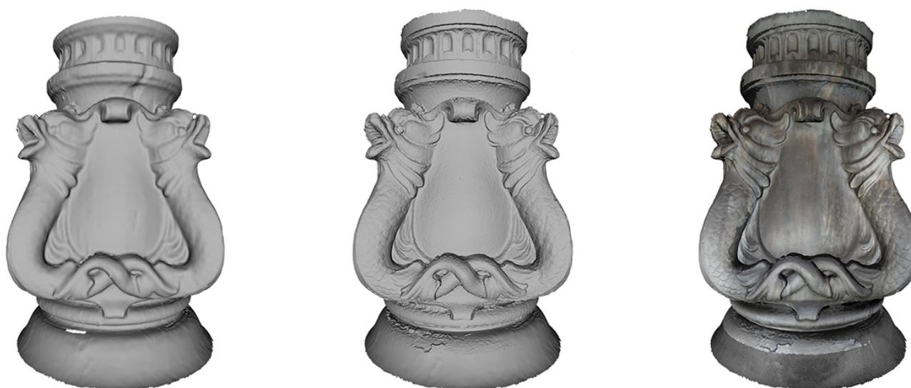
Figure 17. Surface reconstruction of the central baluster of the fountain with the integration between laser scanner and digital photogrammetry.
