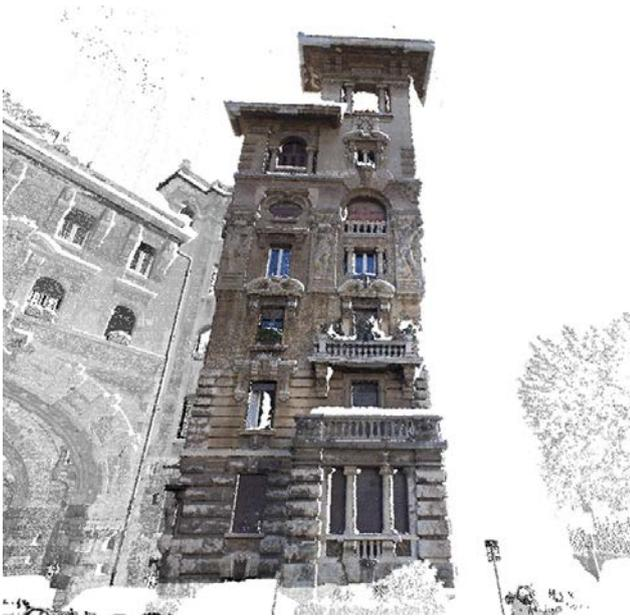
Figure 1. Point cloud from laser scanner of the main façade of an historical building in Rome, Palazzo degli Ambasciatori. The cloud presents different shadow areas generated from the position of the laser.
