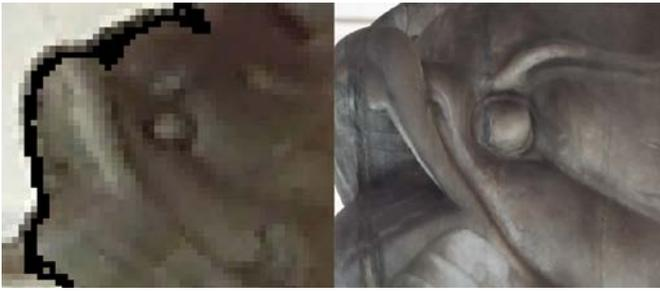
Figure 6. The positioning error of the points depends mainly on the different resolution of the clouds. The eye of the mythological dolphin is represented with more pixels in the image-based acquisition (right) than the laser scanner (left).
