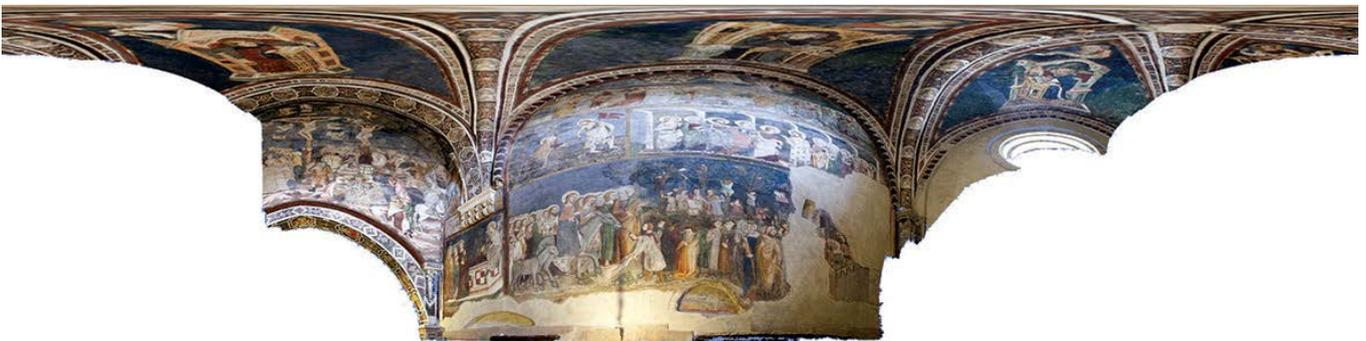
Figure 7. Virtual Scan of the image-based acquisition from a spherical camera positioned in the same projection centre of the laser scanner and with a 360x1800 resolution grid, Monastery of Subiaco.
