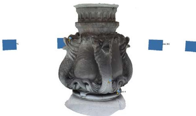
Figure 10. Image-based project of the central baluster of the fountain. Characterized by 4 mythological dolphins the pattern of the marble allowed to pick at least 5 GCPs.
