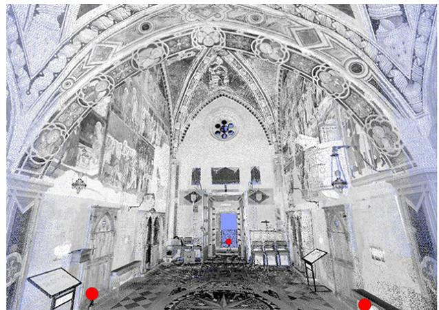
Figure 3. The scans registration phase was usually conducted through planar and/or spherical targets. Planar GCPs are often related to a topographical survey.
