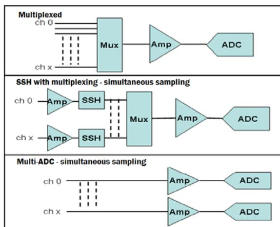
Figure 1. Simultaneous sampling architecture – simultaneous sample and hold (ssh).
