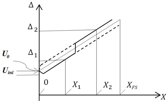
Figure 3. Maximum absolute error vs. input signal for ADC.
