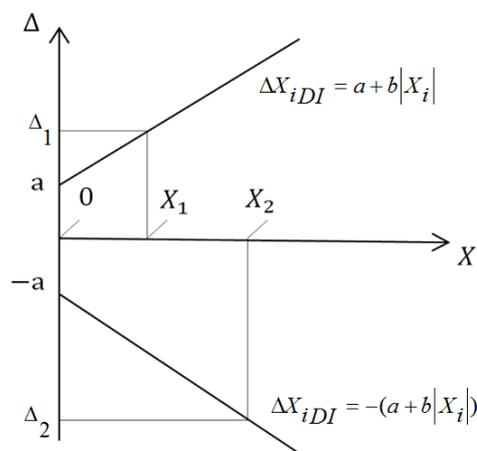
Figure 2. Maximum absolute measurement error vs. input signal for digital instruments.
