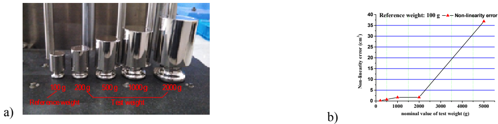
Figure 5. The reference weight of 100 g and test weights ranging from 200 g to 5 kg (a) and the measuring results (b).
