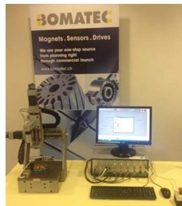
Figure 4. Bomatec AG utilizes the SENIS Magnetic Field Mapping System for quality control of permanent magnets.
