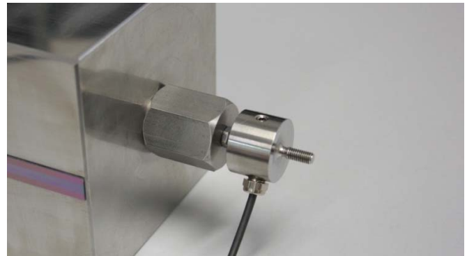
Figure 1. Force transducer HBM U9B / 1 kN mounted at the cube-shaped 10 kg reaction mass of the 20 kN shock force calibration device by means of an adapter with central threads and a counter nut.
