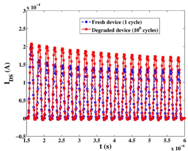
Figure 12. Time-resolved measurement of the drain current  $I_{DS}$  during a short (20x50 ns) programming signal before (circles) and after (squares) short/STD program/erase cycling ( $10^6$  cycles).
