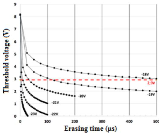
Figure 17. Erasing kinetics for  $-23\text{ V} < V_{pp} < -18\text{ V}$ . “Erased” threshold voltage measured after a standard erasing operation is added for comparison (dotted line).
