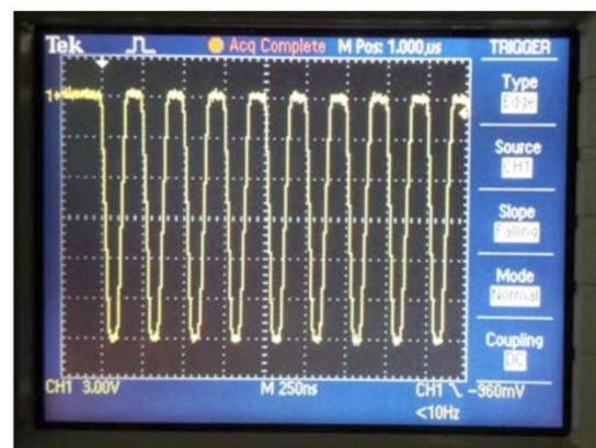
Figure 5. Oscilloscope observation of the control gate signal of a Flash floating gate transistor during a FN erase operation.
