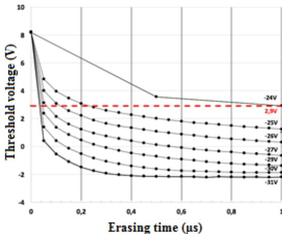
Figure 18. Erasing kinetics for  $-31\text{ V} < V_{pp} < -24\text{ V}$ . “Erased” threshold voltage measured after a standard erasing operation is added for comparison (dotted line).
