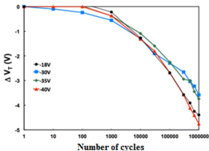
Figure 20. Programming window closure up to  $10^6$  program/erase cycles for various erasing  $V_{pp}$  values (from -30 V to -40 V, with standard -18 V results for comparison). Each measurement point has been averaged over ten Flash memory cells.
