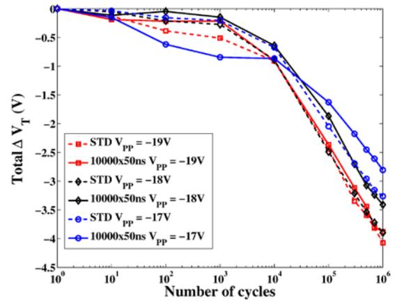
Figure 7. Programming window closure up to  $10^6$  program/erase (STD/STD and STD/Short) cycles for various erasing  $V_{pp}$  values. Each measurement point has been averaged over ten Flash memory cells.
