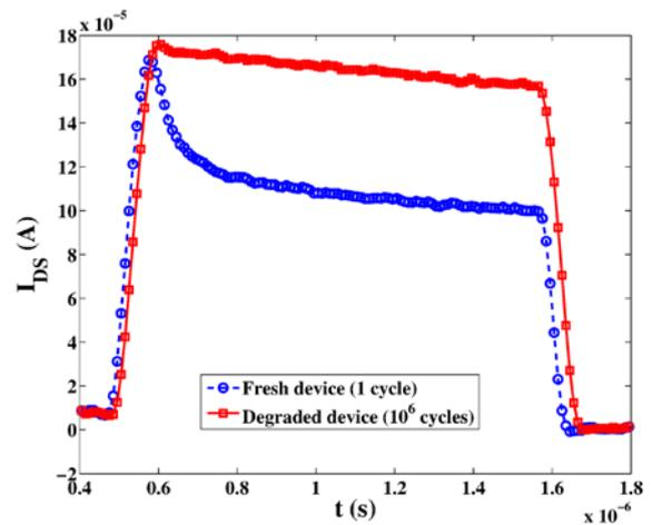
Figure 11. Time-resolved measurement of the drain current  $I_{DS}$  during a standard programming signal before (circles) and after (squares) STD/STD program/erase cycling ( $10^6$  cycles).
