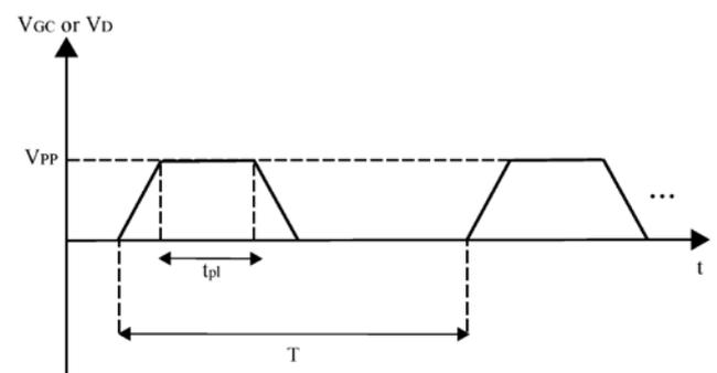
Figure 8. Schematic representation of a period of the electrical signals applied to the control gate ( $V_{Gc}$ ) or drain ( $V_D$ ) of the memory transistor. The duty cycle is calculated as the ratio of the plateau duration  $t_{pl}$  to the period value  $T$ .
