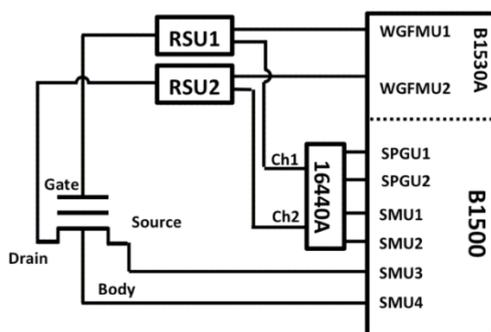
Figure 2. Experimental setup used to perform endurance tests with current consumption measurements.
