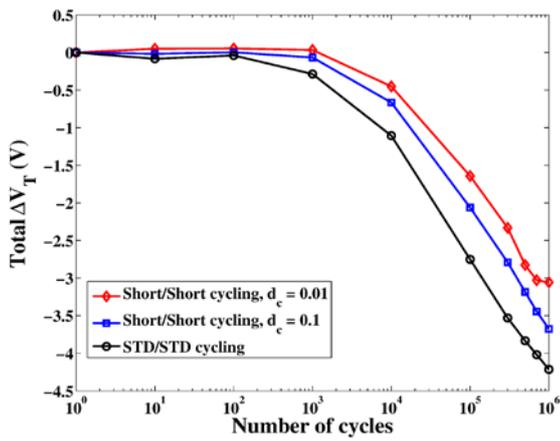
Figure 9. Programming window closure up to  $10^6$  program/erase cycles obtained for various duty cycle values. Each measurement point has been averaged over ten Flash memory cells.
