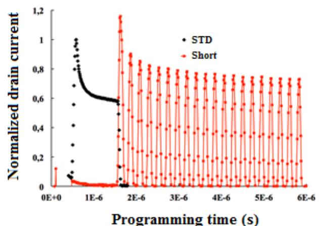
Figure 13. Current consumption measurements during STD (black) and Short (red) programming operations performed on a fresh Flash device.
