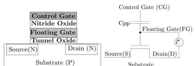
Figure 1. Schematic (left) and electric (right) representation of a Flash floating-gate transistor.
