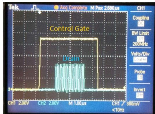
Figure 3. Oscilloscope observation of the control gate (yellow) and drain (blue) signals for a short-pulsed CHE programming of the Flash memory cells.
