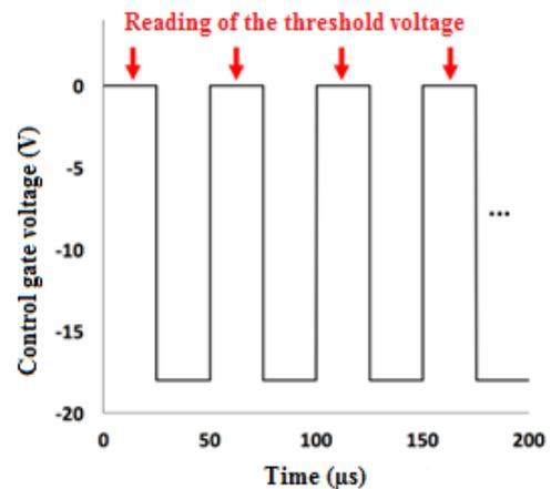
Figure 16. Experimental method to investigate erasing kinetics of the tested Flash cells.
