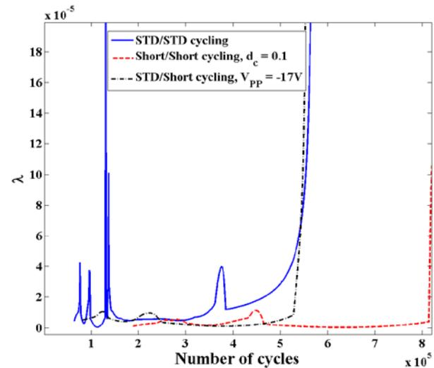
Figure 15. Calculated failure rate of Flash memory cells subjected to STD/STD, Short/Short ( $d_c = 0.1$ ), and STD/Short ( $V_{pp} = -17$  V) cyclings.
