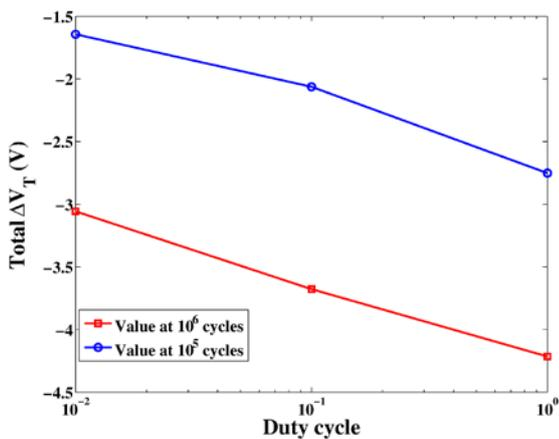
Figure 10. Total window closure as a function of duty cycle obtained from data of Figure 9 at  $10^5$  and  $10^6$  cycles.
