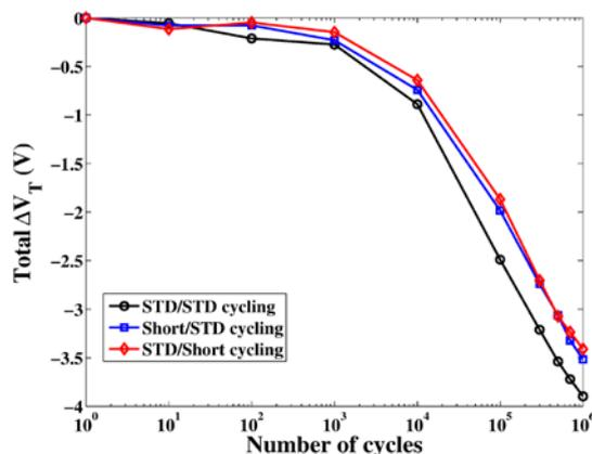
Figure 6. Programming window closure up to  $10^6$  program/erase (STD/STD, Short/STD and STD/Short) cycles. Each measurement point has been averaged over ten Flash memory cells.
