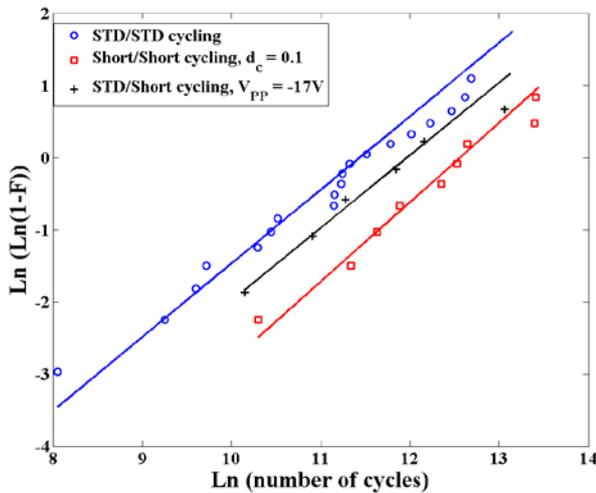
Figure 14. Weibull plot obtained for Flash memory cells subjected to STD/STD, Short/Short ( $d_c = 0.1$ ), and STD/Short ( $V_{pp} = -17$  V) cyclings. The lines displayed in that figure correspond to the fitting of experimental data using Weibull parameters found in table Table 1.
