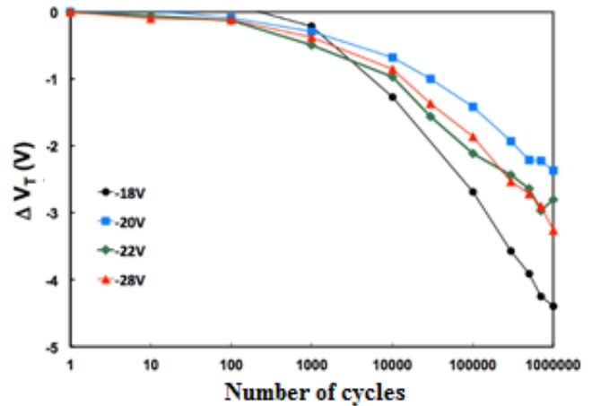
Figure 19. Programming window closure up to  $10^6$  program/erase cycles for various erasing  $V_{pp}$  values (from  $-18\text{ V}$  to  $-28\text{ V}$ ). Each measurement point has been averaged over ten Flash memory cells.
