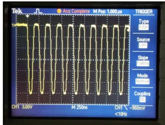
Fig. 5. Oscilloscope observation of the control gate signal of a Flash floating gate transistor during a FN erase operation.
