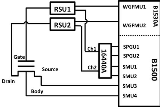
Fig. 2. Experimental setup used to perform endurance tests with current consumption measurements.
