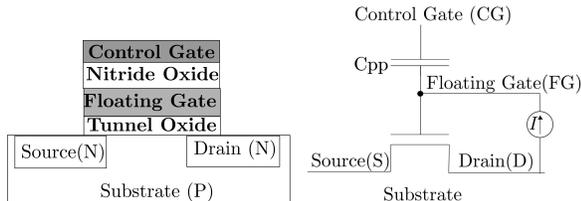
Fig. 1. Schematic (left) and electric (right) representation of a Flash floating-gate transistor.
