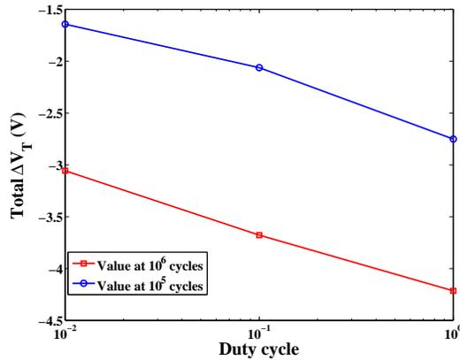
Fig. 10. Total window closure as a function of duty cycle obtained from data of Fig.9 at  $10^5$  and  $10^6$  cycles.
