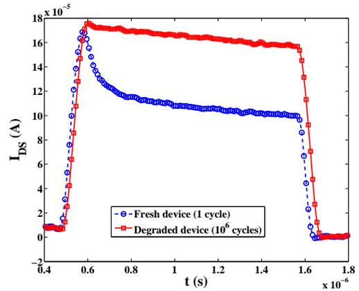
Fig. 11. Time-resolved measurement of the drain current  $I_{DS}$  during a standard programming signal before (circles) and after (squares) STD/STD program/erase cycling ( $10^6$  cycles).
