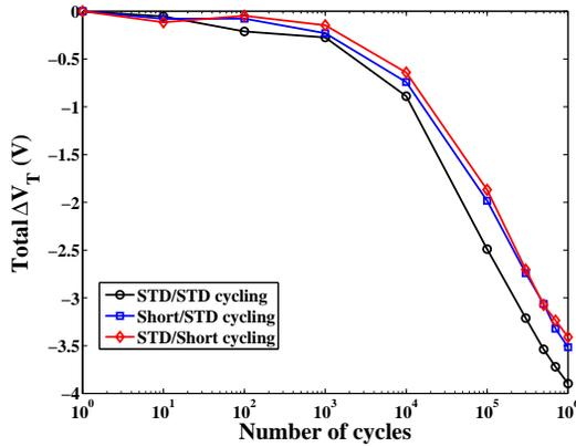
Fig. 6. Programming window closure up to  $10^6$  program/erase (STD/STD, Short/STD and STD/Short) cycles. Each measurement point has been averaged over ten Flash memory cells.
