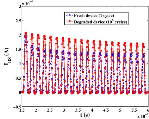
Fig. 12. Time-resolved measurement of the drain current  $I_{DS}$  during a short ( $20 \times 50$  ns) programming signal before (circles) and after (squares) short/STD program/erase cycling ( $10^6$  cycles).
