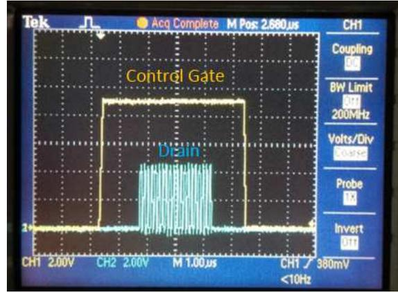
Fig. 3. Oscilloscope observation of the control gate (yellow) and drain (blue) signals for a short-pulsed CHE programming of the Flash memory cells.
