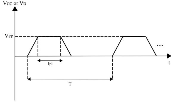
Fig. 8. Schematic representation of a period of the electrical signals applied to the control gate ( $V_{GC}$ ) or drain ( $V_D$ ) of the memory transistor. The duty cycle is calculated as the ratio of the plateau duration  $t_{pl}$  to the period value  $T$ .
