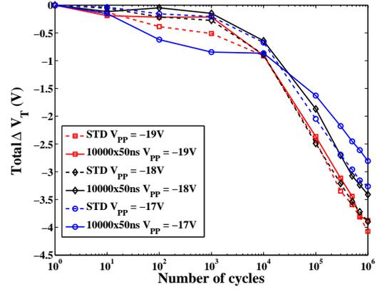
Fig. 7. Programming window closure up to  $10^6$  program/erase (STD/STD and STD/Short) cycles for various erasing  $V_{PP}$  values. Each measurement point has been averaged over ten Flash memory cells.
