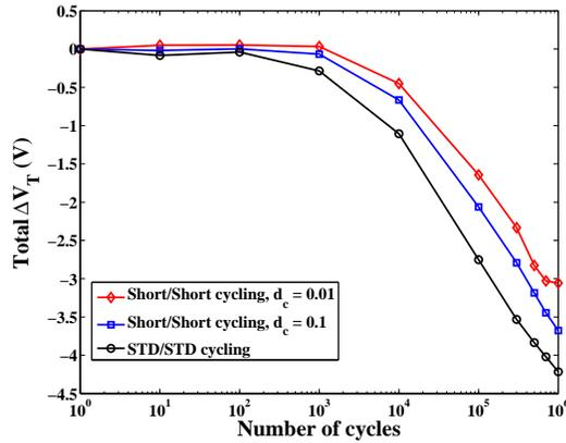
Fig. 9. Programming window closure up to  $10^6$  program/erase cycles obtained for various duty cycle values. Each measurement point has been averaged over ten Flash memory cells.
