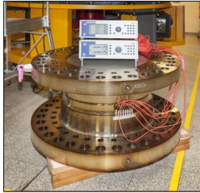
Figure 4. 5 MN·m torque transducer together with two DMP41 bridge amplifiers for the readout of the 8 channels of the transducer.
