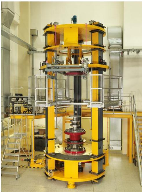
Fig. 2. The 1.1 MNm Standard Calibration Machine of PTB.
