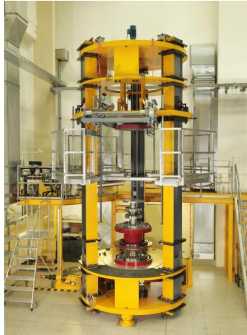
Figure 2. Standard Torque Calibration Machine for nominal torques up to 1.1 MN·m.
