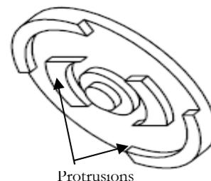
Figure 3. Universal rotating cap lower side.
