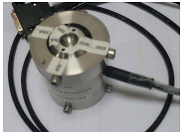
Figure 13. Manufactured multi-capacity load cell without loading plate.
