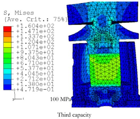
Figure 7. Results of FE stress due to 15 kN load on 3<sup>rd</sup> range.
