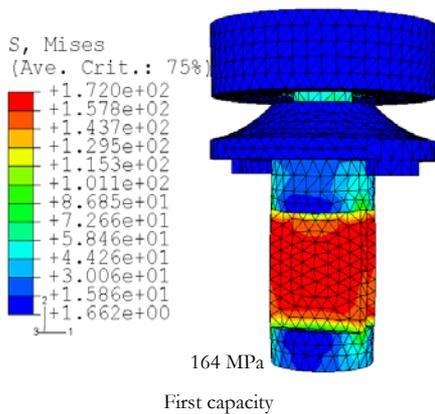
Figure 5. Results of FE stress due to 15 kN load on 1<sup>st</sup> range.
