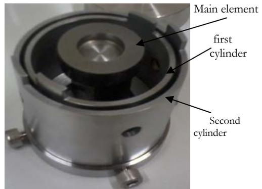
Figure 8. Main parts assembly.
