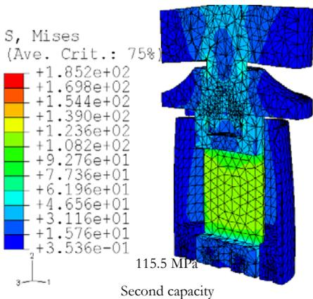
Figure 6. Results of FE stress due to 15 kN load on 2<sup>nd</sup> range.
