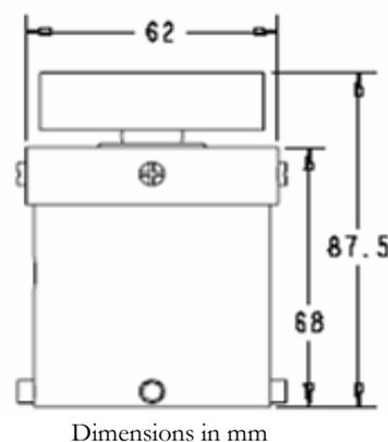
Figure 4. Load cell overall dimensions.
