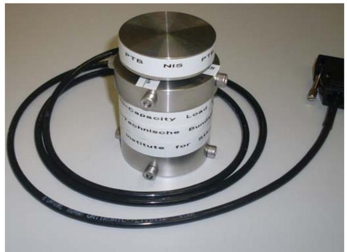
Figure 12 . Manufactured multi-capacity load cell with loading plate.
