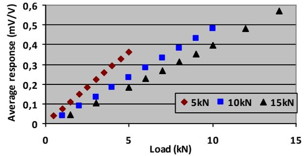
Figure 9. Representative graph for the average response for the three capacities at maximum load.
