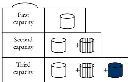
Figure 1. Schematic of the concept of adding elastic elements to form a three-range multi-capacity load cell.
