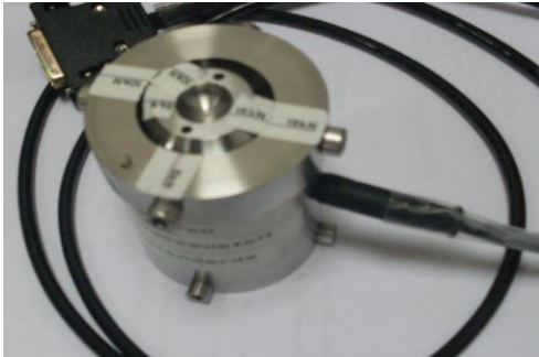
Fig. 8. Manufactured multi-capacity load cell without loading plate
