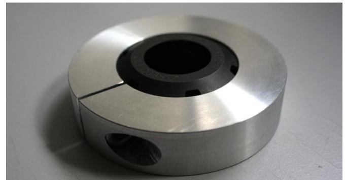
Figure 9. Moment of inertia element J \approx 300 \text{ kg} \cdot \text{mm}^2 mounted on a clamping nut.
