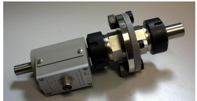
Figure 8. Torque transducer HBM T5 (left) with the mass moment of inertia element J \approx 900 \text{ kg} \cdot \text{mm}^2 (right).
