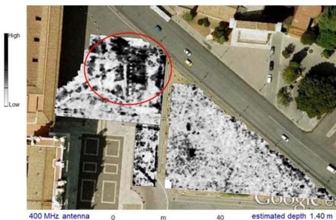
Figure 5. St. John Lateran square. GPR time slices in the time window 58-61 ns twt (estimated depth 1.4 m) for the 400 MHz antenna.
