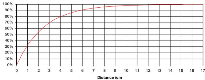
Figure 23. Plot showing the decrease of the magnetic effects versus the increase in the distance to the source of the electromagnetic fields as a function of expression (11).
