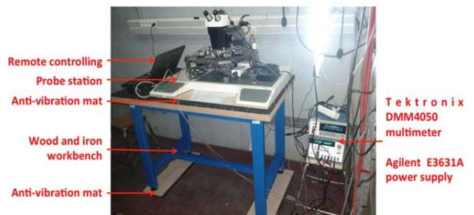
Figure 6. Picture of the proposed test bench, embedded in the low-noise environment.
