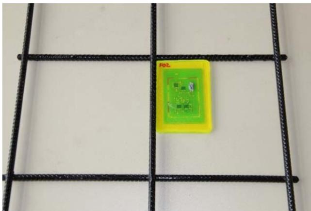
Figure 3. Encapsulated RFID sensor tag with reinforcement.
