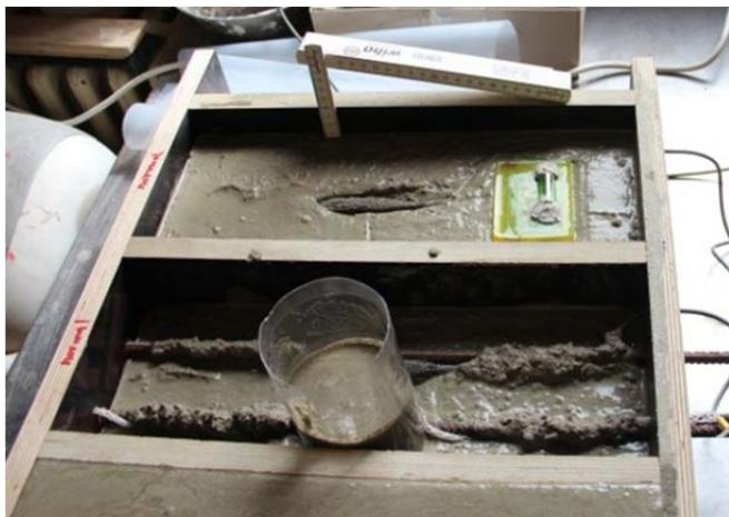
Figure 4. Preparation of concrete specimen with embedded RFID sensor tag.
