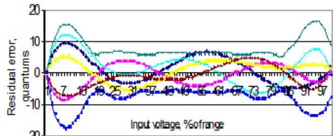
Figure 4. Residual error vs input voltage for ADC noise  $\pm 6$  quanta.
