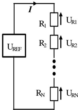
Figure 1. Circuit of  $N$ -resistors voltage divider.
