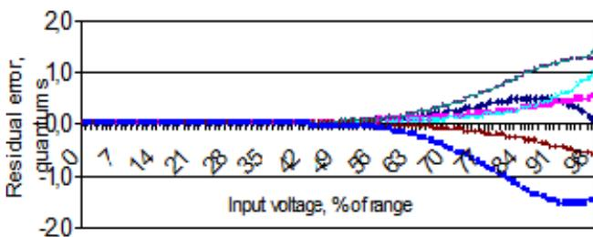
Figure 3 Residual error vs input voltage for resistors' error  $\pm 1$  %.
