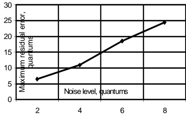
Figure 5. Maximum residual error vs ADC noise level.
