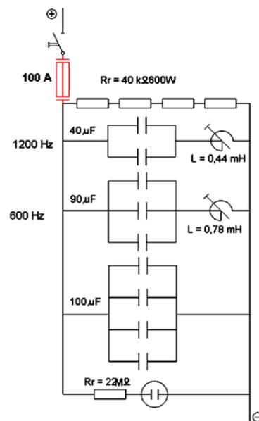
Figure 1. A simplified scheme of a filter with two resonance contours (600 and 1200 Hz) used in 12-pulse 3 kV DC traction substations.
