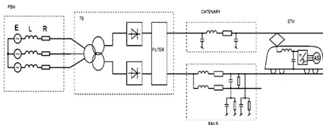
Figure 2. A scheme of a circuit of electrical energy delivery from an AC power supply network (PSN) to a rectifier traction substation with a DC side filter and via catenary to an electric vehicle (EV).
