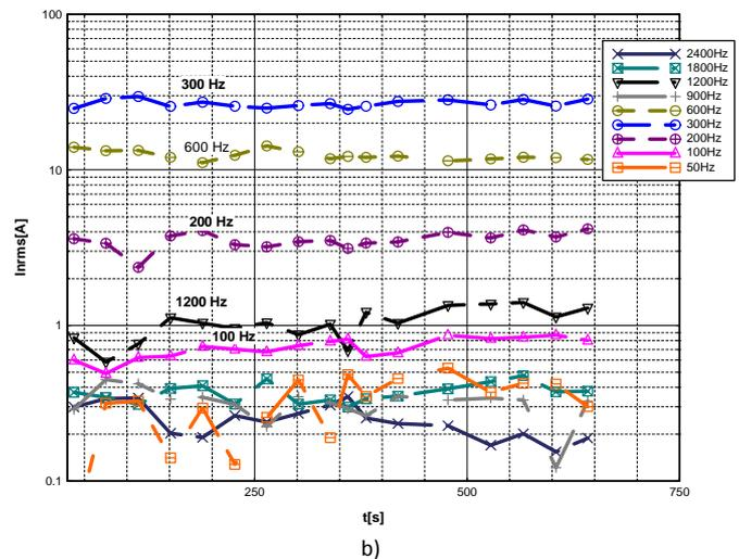
Figure 5. Rms values of higher harmonics of substation's filter current a) with a resonance filter, b) with a resonance filter and an expanded aperiodic element from 100 to 350  $\mu\text{F}$ .
