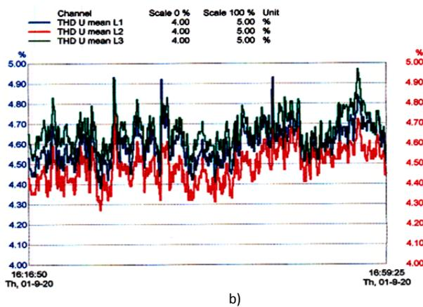
Figure 3. The level of higher harmonics in a 15 kV line that operates in the idle state, participation (of individual voltage harmonics a) THD U in particular phases-b).
