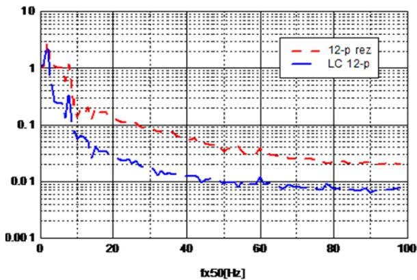
Figure 8. Comparison of attenuation characteristic (4) of a thereto used resonance filter (signed as: 12-p rez) with a 12-pulse unit and LC filter (LC 12-p), noticeably better attenuation of a LC filter with the supply of a substation with distorted and asymmetric voltage, when 300 Hz harmonic is present.
