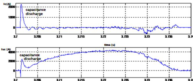
Figure 6. Short-circuit current  $I_{sc}$  at the output of a 3 kV DC traction substation (lower figure) and capacitance of a filter's current  $-I_c$  (upper figure) – the observed peak current is caused by a sudden capacitance discharge.
