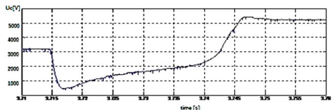
Figure 7. Voltage  $U_c$  at capacitance terminals during a short-circuit clearing.
