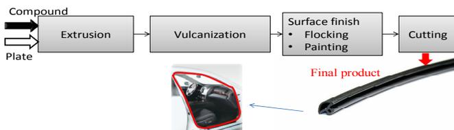
Figure 1. Stages for the rubber manufacturing.
