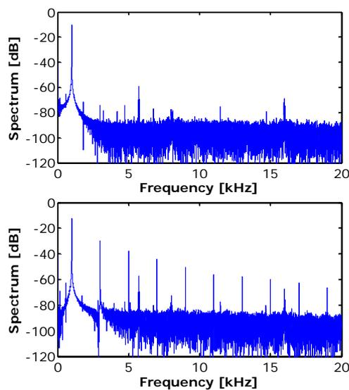
Figure 14. Example of FFT calculation done within the data acquisition device. Sinusoidal signal (top) and triangular signal (bottom).
