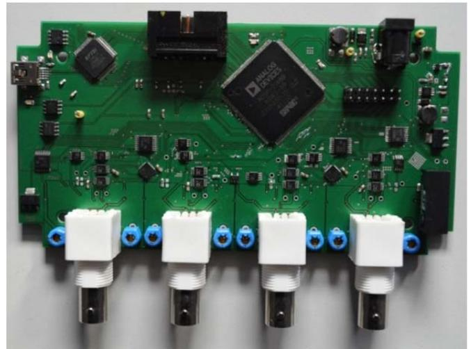
Figure 7. Implemented system. The final PCB has 145 mm length and 75 mm width.
