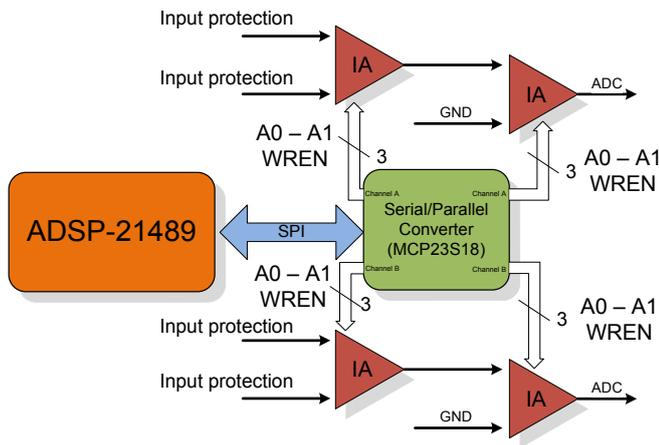
Figure 5. Detail of gain programming stage.
