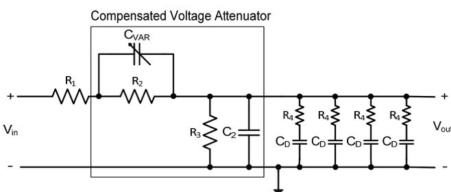
Figure 3. Equivalent analog input circuitry for single-ended acquisitions.
