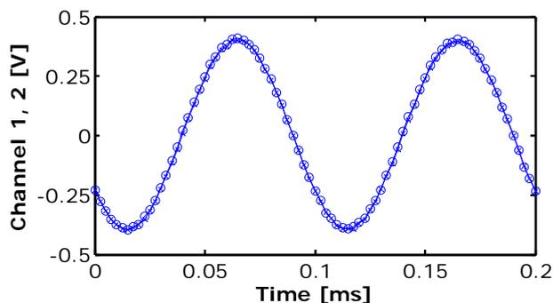
Figure 12. Simultaneous acquisition of a 10 kHz signal. Both channels are represented (the channel 1 samples are the circles and the samples from channel 2 are the crosses).
