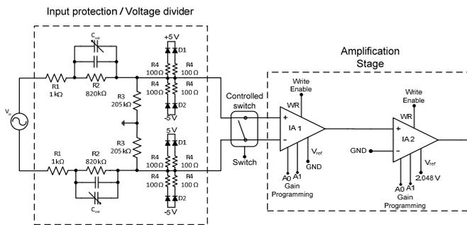
Figure 2. Analog signal conditioning circuit.
