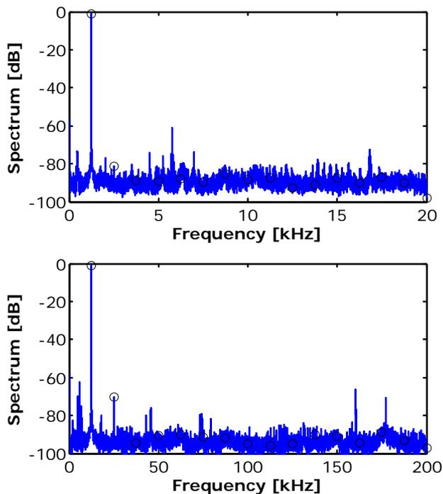
Figure 11. Measured average spectrum THD measurements. The circles represent the detected harmonic amplitudes. The top spectrum corresponds to a 1250 Hz sine signal acquired at 40 kS/s and the resulting THD is -79 dB. The bottom spectrum corresponds to a 12.5 kHz sine signal acquired at 400 kS/s and the resulting THD is -72.1 dB.
