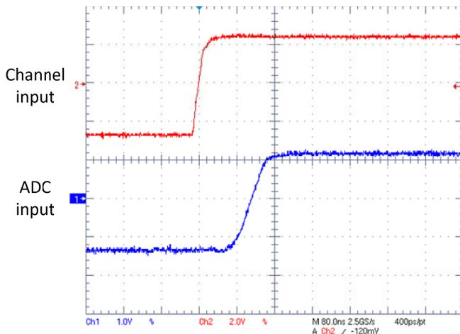
Figure 9. Delay/rising time measurement.
