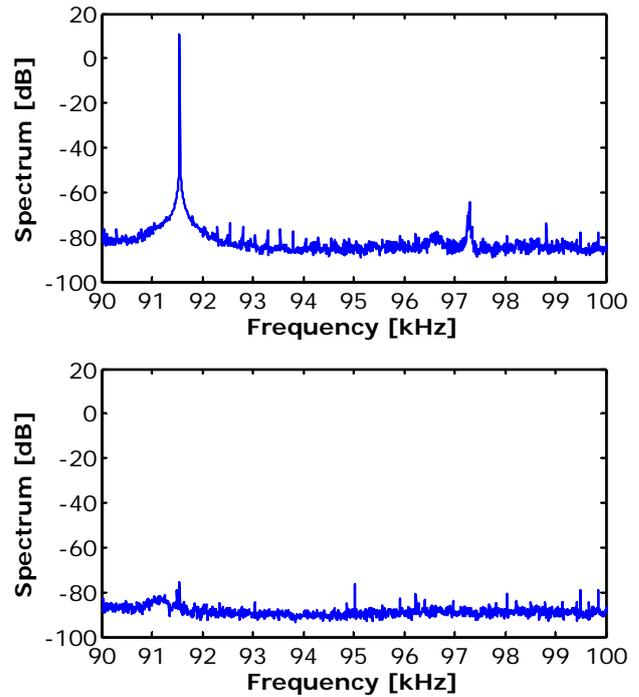
Figure 10. Measured average spectrum cross-talk measurements for 91.5523 kHz. The top average spectrum represents the input sinusoidal signal while the bottom average spectrum is the one obtained on the non-stimulated channel.
