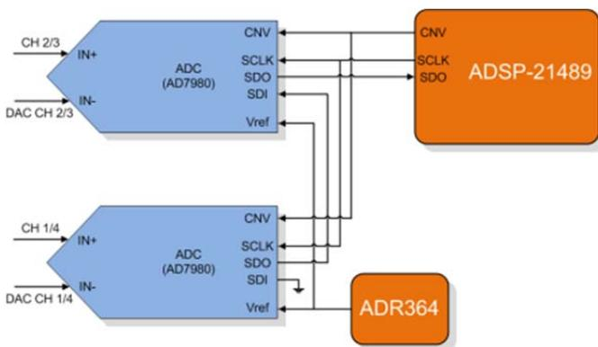
Figure 6. ADC daisy-chain connection. Each pair of ADCs shares the same SPI connection to the DSP.
