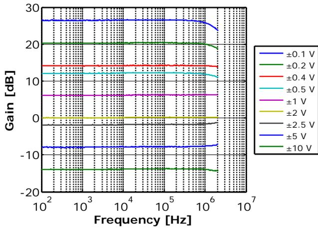
Figure 8. Input frequency responses for all ranges in one channel. The results for the other channels are identical.
