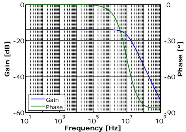
Figure 4. Simulation results of the gain of the analog input circuit before the ADC.
