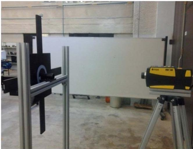
Figure 1. Mutual position between LDV and fold mirrors structure.
