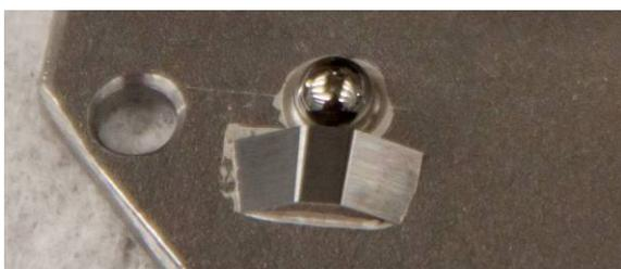
Figure 5. Calibration sphere and angled flats.
