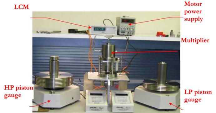
Figure 7. Multiplier system test setup.
