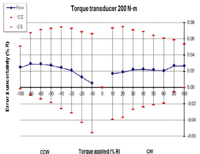
Figure 7. Error and uncertainty of the 200 N-m torque transducer.
