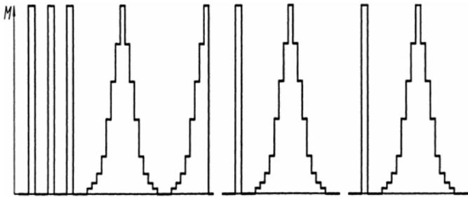
Figure 2. Example of the calibration procedure at 0°, 120° and 240° mounting positions for classes 0.05 and 0.1 (DIN 51309:2005).
