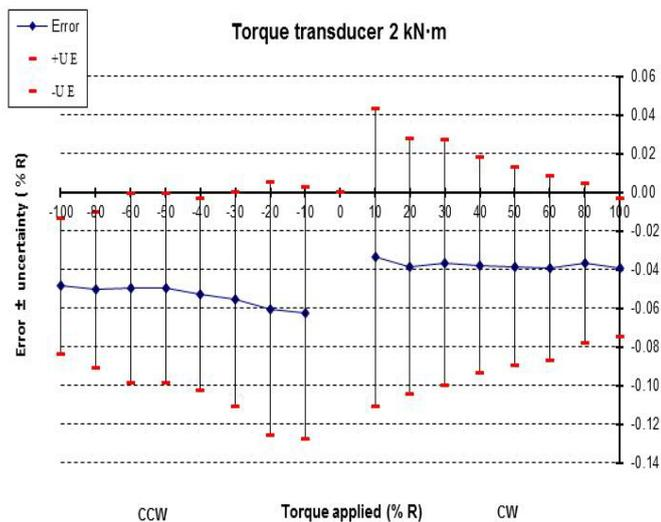
Figure 8. Error and uncertainty of the 2 kN·m torque transducer.
