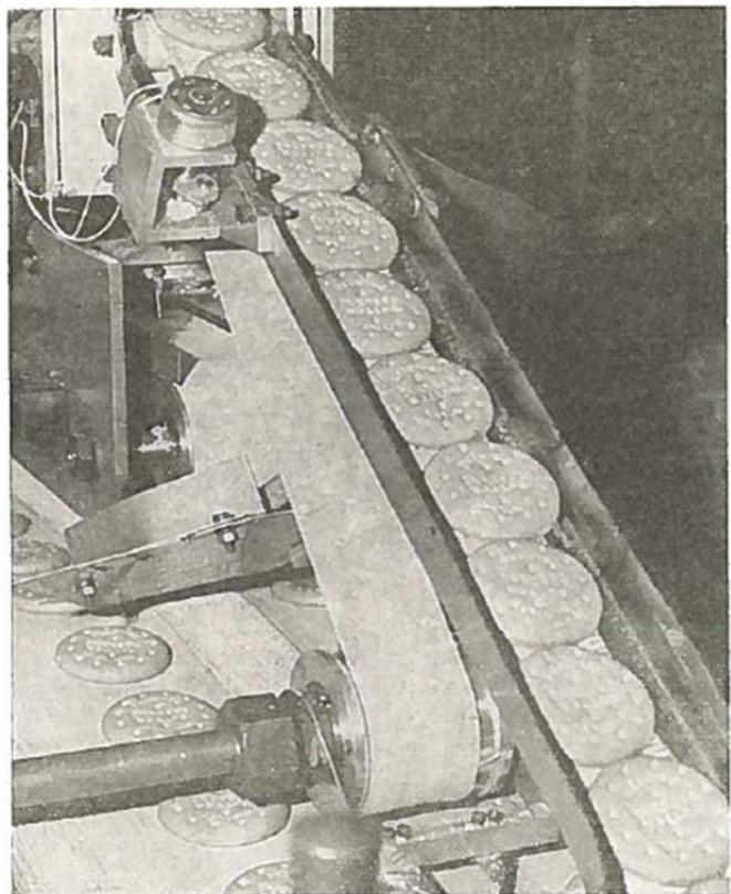
Figure 1. Automatic sampling machine installed on a biscuit line.
