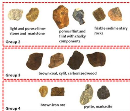
Figure 9. Particular components of mineral aggregates to be considered.
