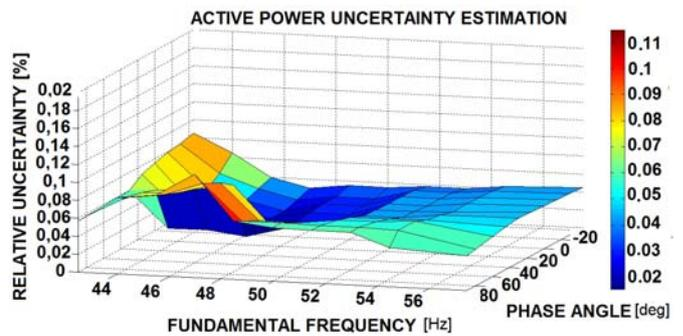
Figure 14. Active Power Uncertainty Estimation vs phase angle and fundamental frequency.
