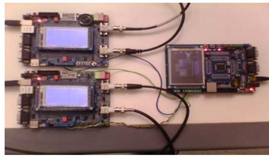
Figure 18. Example of device connection for data transmission.
