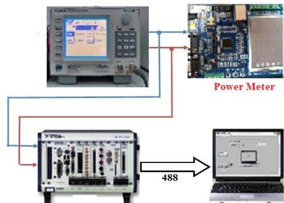
Figure 12. Experimental set-up for static characterization.
