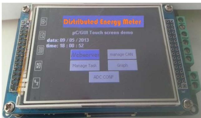
Figure 8. User interface for accessing to the implemented tasks.
