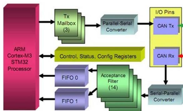
Figure 7. CAN communication device architecture.
