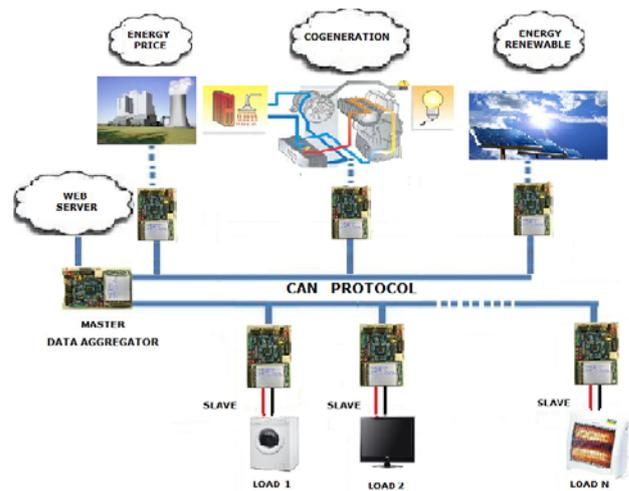
Figure 1. Architecture of the proposed smart metering network.
