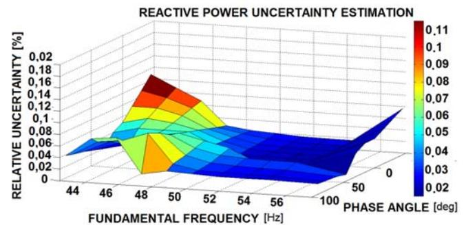
Figure 15. Reactive Power Uncertainty Estimation vs phase angle and fundamental frequency.
