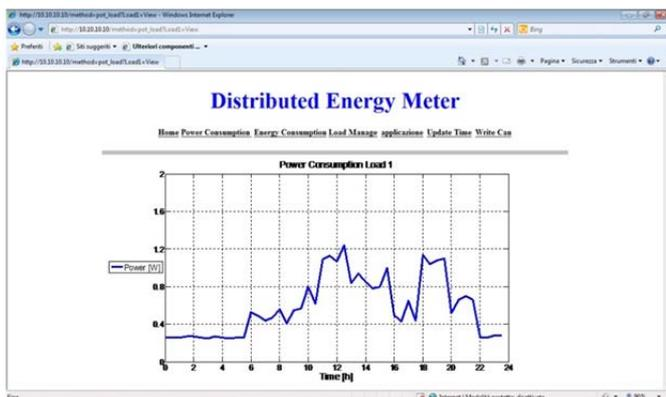
Figure 11. Power graph of a specific load.
