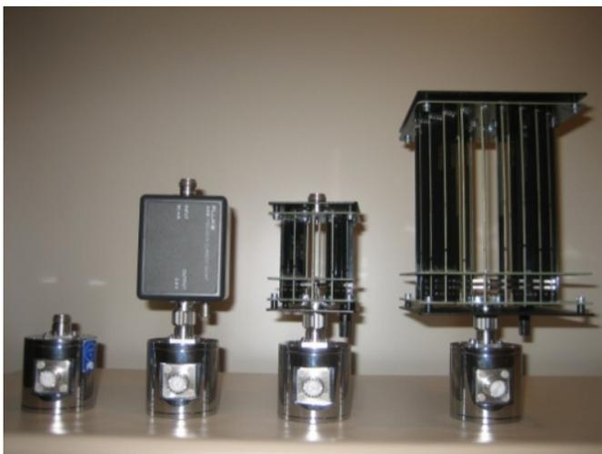
Figure 6. ac-dc current transfer standards.
