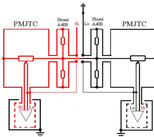
Figure 2. ac-dc current transfer with potential driven guards (PMJTCs with shunts for current ranges above 10 mA).
