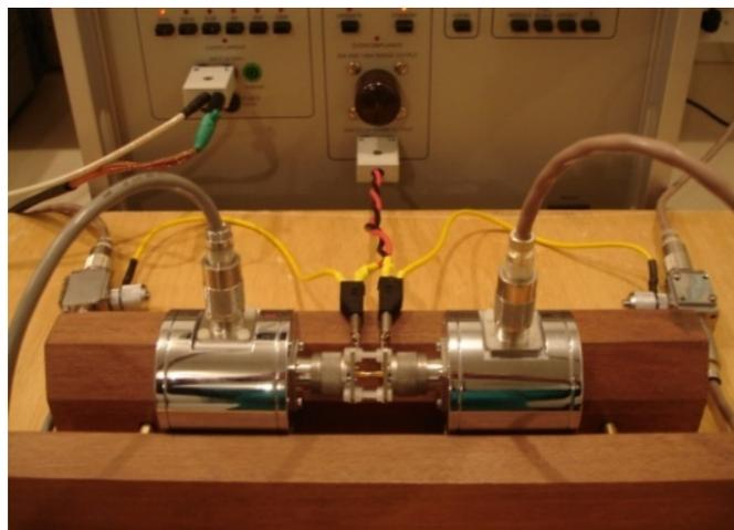
Figure 4. Connection of the ac-dc current transfer standards in series.
