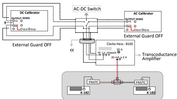
Figure 1. Measurement set-up for ac-dc current transfer difference measurements.
