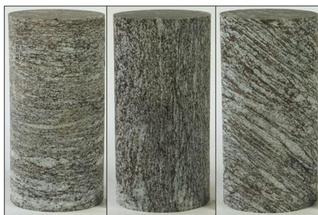
Figure 2. Test specimens with a slenderness ratio of 2:1, drilled in three different directions (K, P, and S) in relation to the metamorphic foliation (left – K specimen, in the middle – P specimen, right – S specimen).
