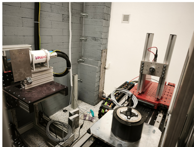
Figure 3. Experimental configuration employing a high-power X-ray source and a large-area scintillator-coupled detector for large-field-of-view XCT imaging.
