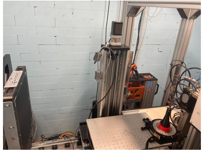
Figure 1. Experimental configuration employing a high-power liquid-metal anode X-ray source and a large-area low-noise flat-panel detector.
