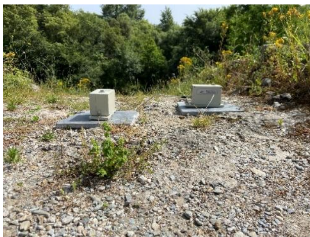
Figure 6. Details of installed seismometers. The stone elements on which the sensors were positioned, acting as support base, guarantee a perfect sensor stability and the quality of the measurements.
