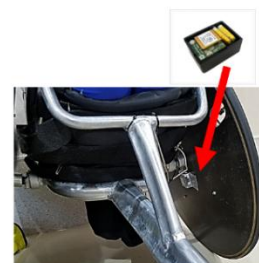
Figure 1. System configuration and IMU specifications. (A) Overview of the Sensor-in-Glove System (SIGS). One IMU (IMU1) is embedded in the glove to record hand motion, while a second IMU (IMU2) is mounted on the wheel to capture wheel rotation. Both IMUs transmit data wirelessly to a PC, and a pulse generator is used for synchronisation. (B) Specifications of the two IMUs used in this study.
