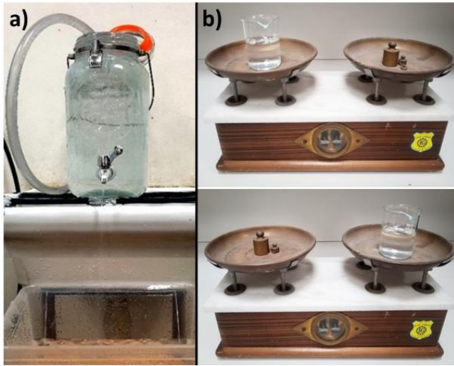
Figure 4. a) Hydraulic apparatus for water-clock time measurements. b) Balance used to assess the accuracy of mass measurements achievable in Galileo's time.
