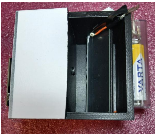
Figure 2. The custom 3D-printed enclosure integrating the imaging and deposition system.
