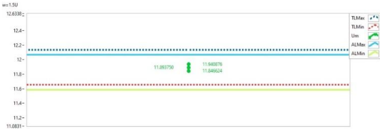
Figure 9. Measured result at a calibration point along the vertical axis 2 V/Div voltage base for UUT1 (Channel 3) for w=1,5U.
