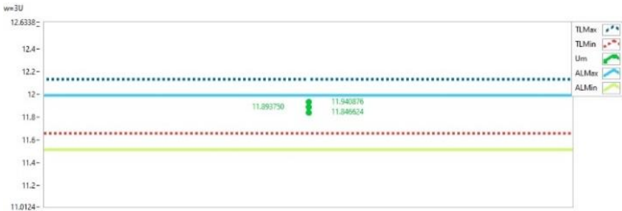
Figure 10. Measured result at a calibration point along the vertical axis 2 V/Div voltage base for UUT1 (Channel 3) for w = 3 U.
