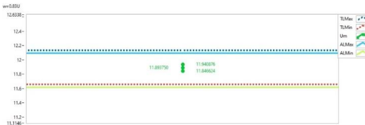
Figure 7. Measured result at a calibration point along the vertical axis 2 V/Div voltage base for UUT1 (Channel 3) for w = 0.83 U .
