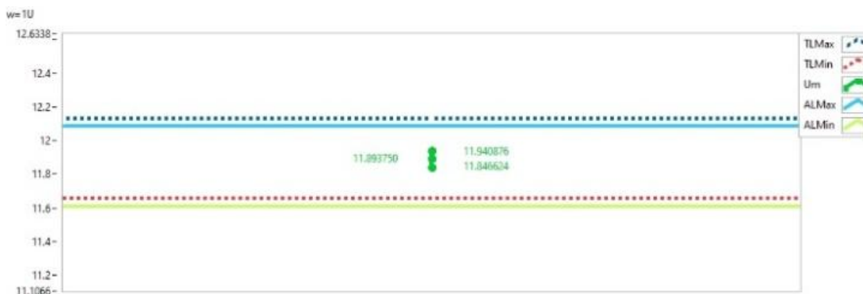
Figure 8. Measured result at a calibration point along the vertical axis 2 V/Div voltage base for UUT1 (Channel 3) for w = U .
