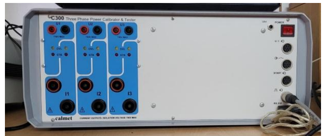
Figure 1. Power calibrator, a secondary RS of LEM, used as a source of harmonically distorted signals and as a reference fundamental reactive power unit.
