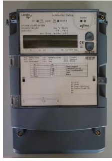
Figure 2. A reactive energy electricity meter with a measuring algorithm based on phase displacement of input voltages by 90° .
