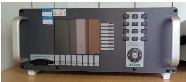
Figure 3. Energy comparator, the primary RS of LEM, with a measuring algorithm based on time displacement of input currents by T/4.
