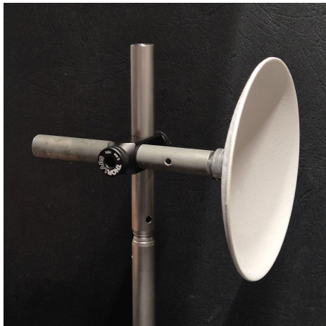
Figure 10. Example of a 3D-printed PLA parabolic reflector (diameter 100 mm) coated with a BaSO 4 -based suspension applied by airbrushing. The multilayer process with intermediate acrylic binder yielded a uniform, matte, and diffusively reflective surface.
