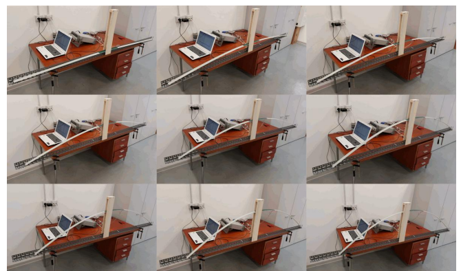
Figure 11. Bench realized for the acquisition of experimental results. The guide with nine fixed positions forces the batten at repeatable curvatures.
