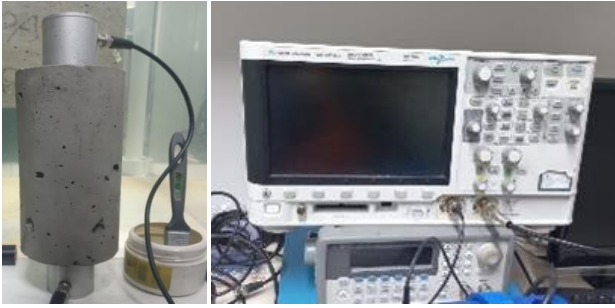
Figure 3. Measurement of the specimen to obtain the ultrasonic velocity.
