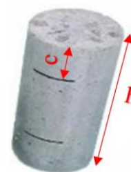
Figure 2. Demonstration of how to mark the test specimens.
