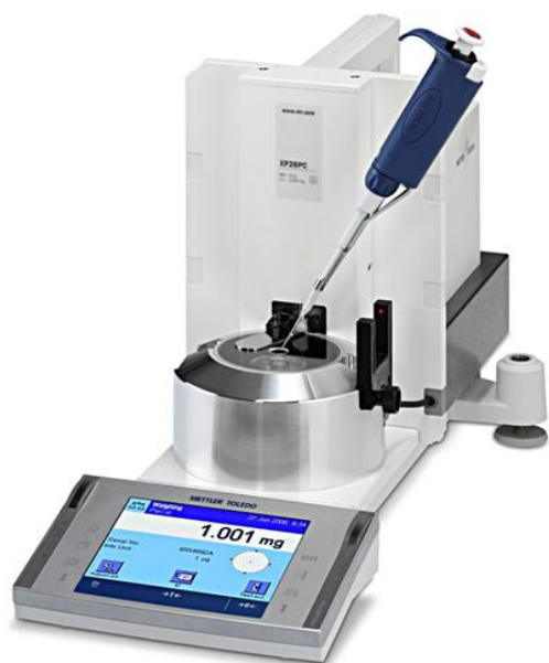
Figure 3. Air saturation system of the Mettler Toledo scale model XP26PC. Operating temperature (20 \pm 1) °C; scale resolution 0.001 mg; measurements in \mu L.
