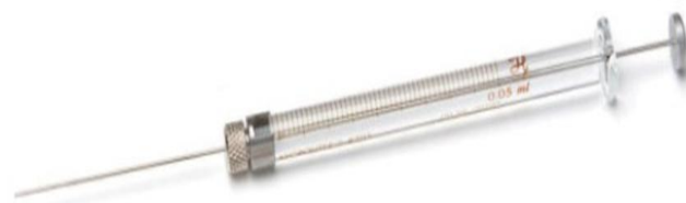
Figure 1. Illustration of a microsyringe, commonly used for precise measurement and dispensing of microvolumes in laboratory applications. This device provides accurate volume control, particularly in the range of 0.1 to 1 \mu\text{L} .
