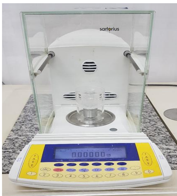
Figure 2. Air saturation system of the Sartorius Genius ME215P. This system has an external acrylic body and a stainless steel interior, with an acrylic weighing container. Operating temperature (20 \pm 1) °C; scale resolution 0.01 mg.
