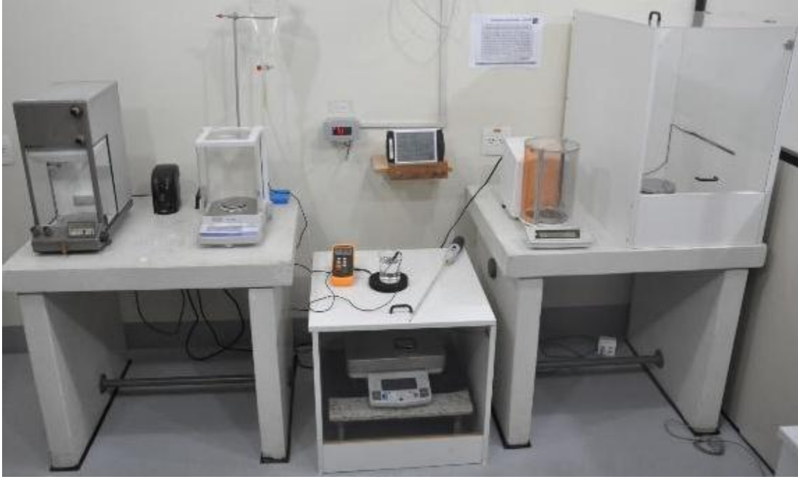
Figure 4. Photograph of the Volume Calibration Laboratory facilities with the bench where the experimental apparatus for measuring microvolume is located, including the scale used for measurements and the instrumentation for monitoring environmental conditions. Temperature (°C) and Humidity (%) monitors visible in setup.
