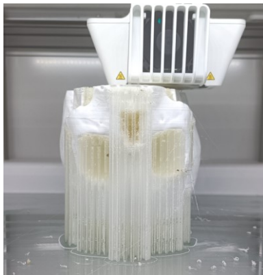
Figure 3. Cranial model 3D printing with UltiMaker S5 Pro Bundle.
