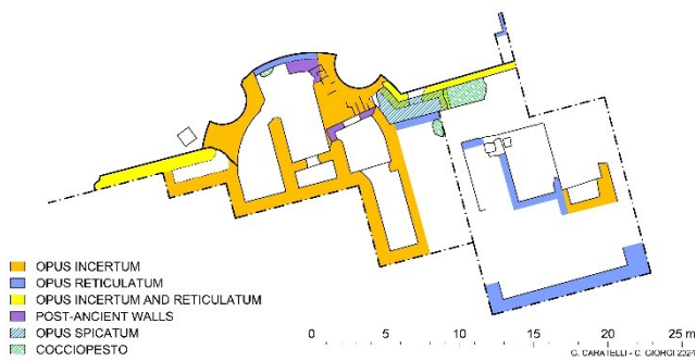
Figure 3. Villa of Gradola. New planimetry from CNR survey indicating the construction technique (in orange opus incertum , in blu opus reticulatum , in yellow opus incertum and reticulatum , in purple post-ancient walls, in light blue dotted opus spicatum , in green dotted cocciopesto ).
