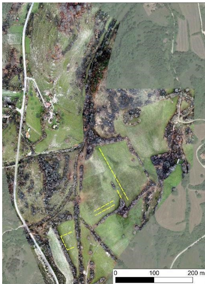
Figure 6. Piano di Santa Croce. Orthophoto generated from the 3D model derived from proximal remote sensing. Indication of identified anomalies in yellow dashed lines.
