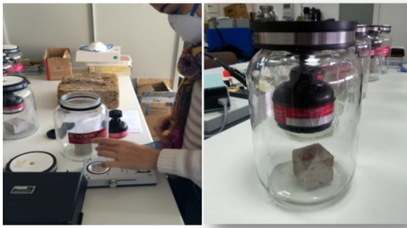
Figure 2. Set up of the electret ion chamber.
