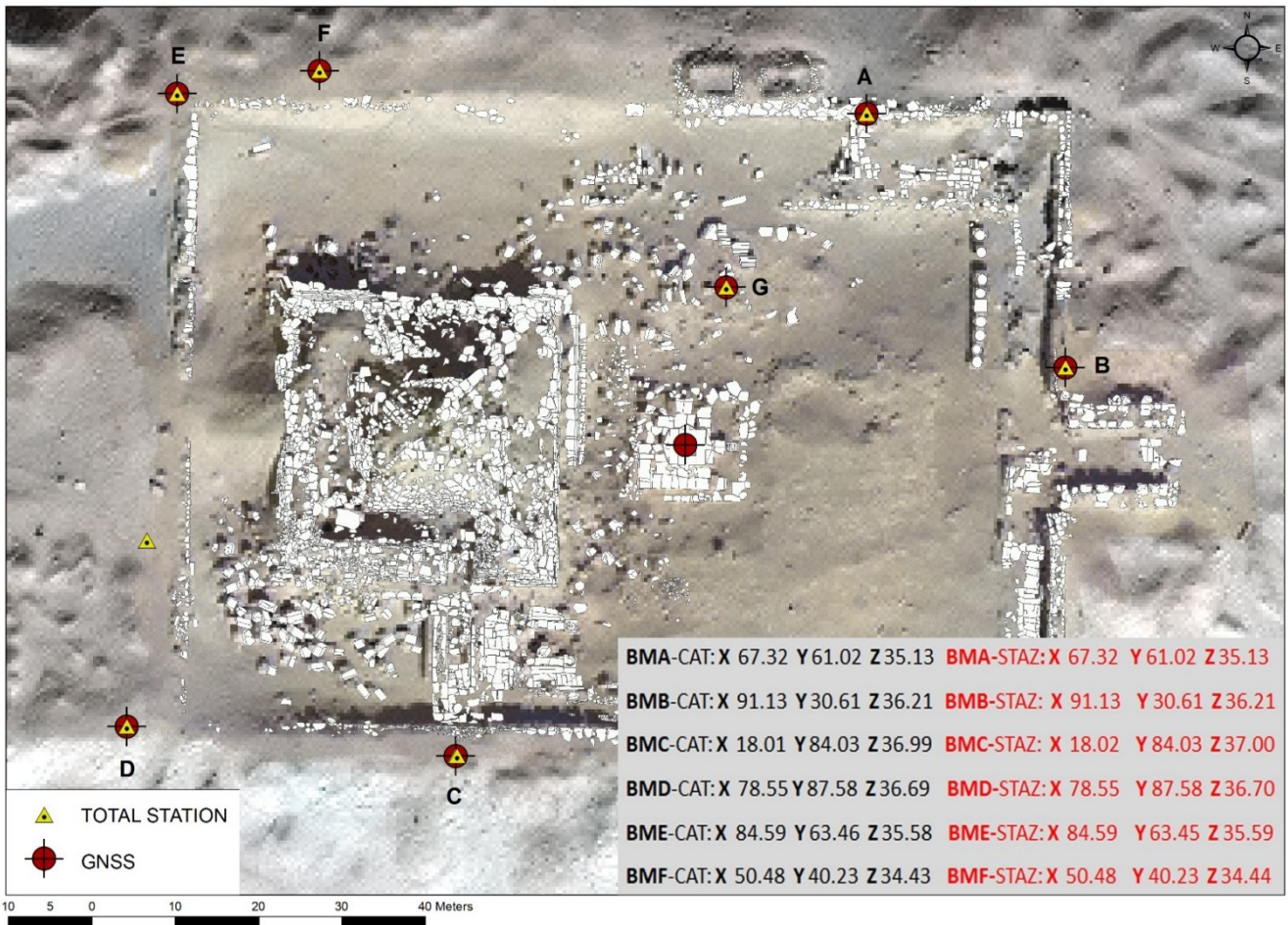
Figure 9. Comparison between surveyed measures by Catalyst DA2 and Total Station (only last 2 integer coordinates numbers are reported while decimal values are rounded to two digits).
