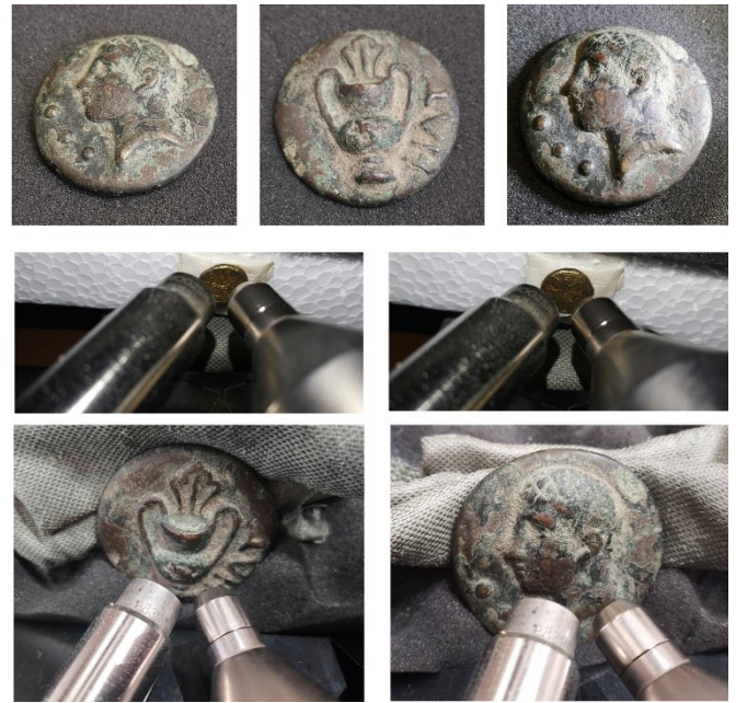
Figure 4. XRF analysis conducted on the two archaeological coins selected for this study and characterized by the typical patinas of copper alloy artifacts.
