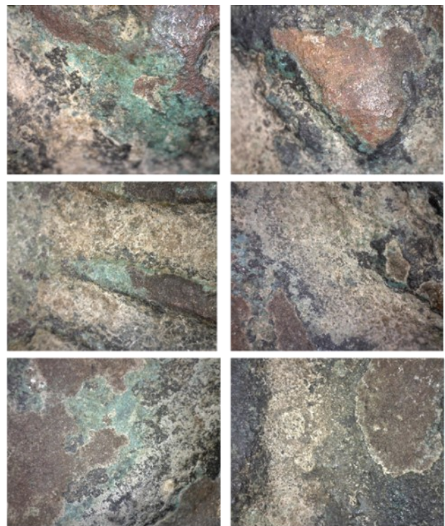
Figure 11. The microscopy on the bronze coin reveals a first reddish-brown layer that is commonly attributed to the formation of copper oxides (cuprite), upon which greenish-blue layers of copper compounds (chlorides or carbonates) subsequently started to grow due to the conservative conditions to which the artifact has been exposed.
