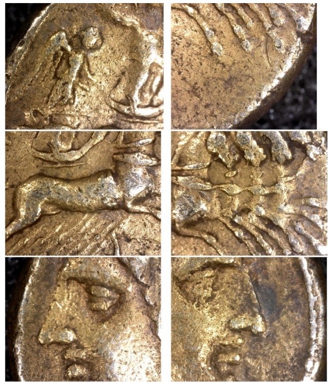
Figure 10. Microscopies of the golden coin revealed abrasions and damage, as well as the formation of corrosion products of the metals present in the alloy (likely silver sulphides and copper oxides).
