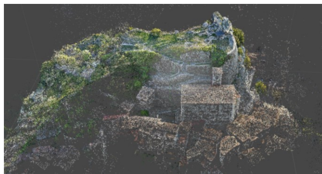
Figure 1. Three-dimensional reconstruction process in Agisoft Metashape: sparse point cloud.
