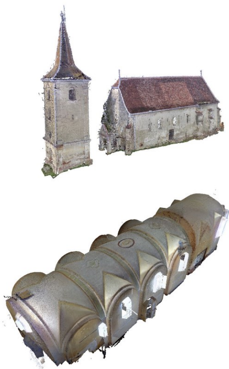
Figure 5. 3D point cloud of the church.
