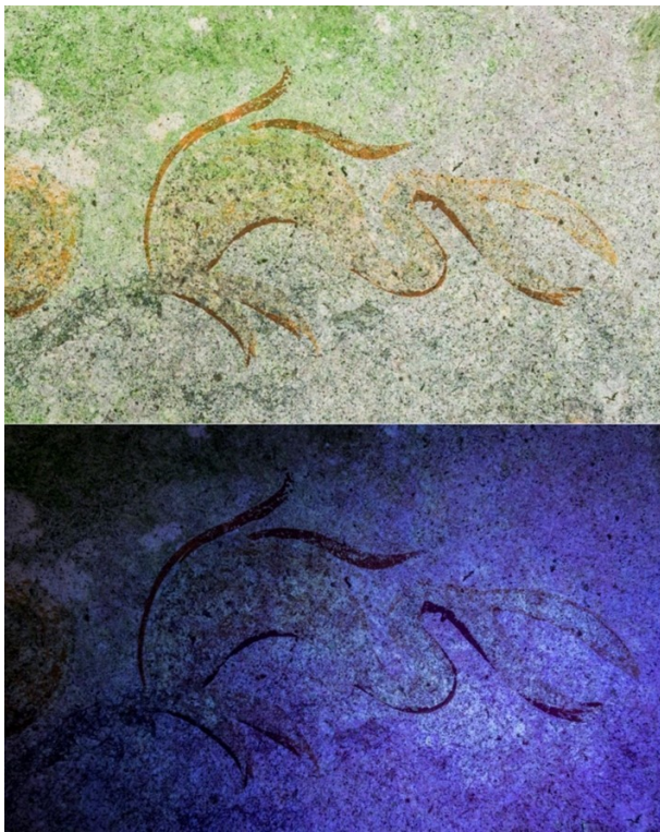
Figure 3. Detail of mural painting, partially covered with biofilm. Top is taken with natural light; bottom is fluorescent after exposition to UV light, obtained using a portable UV lamp (395 nm, Eletrot).
