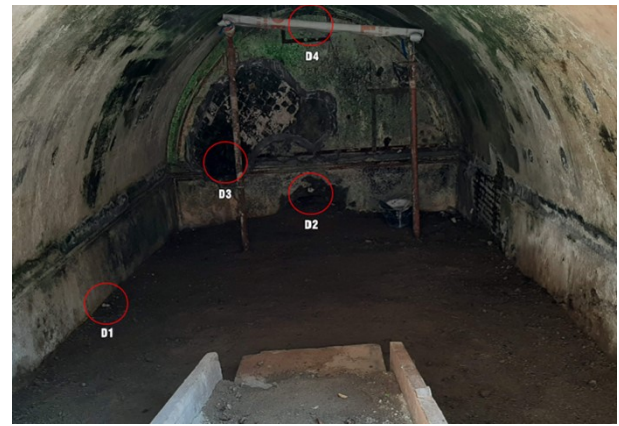
Figure 4. Position of the datalogger for the registration of microclimatic parameters.
